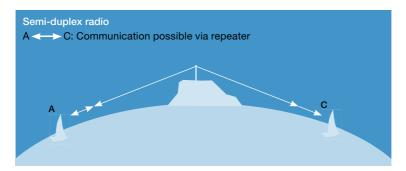
Because VHF signals will not pass through land masses, a repeater may be placed on a hilltop so that stations on opposite sides can communicate with each other. By elevating the repeater station, vessels up to about 70 miles apart can communicate, even though the line of sight between the vessels may be less than 10 miles.
